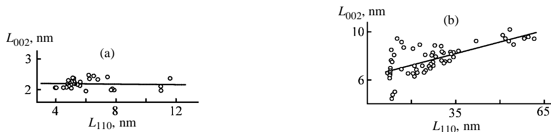
Fig. 1. Correlation of L_{002} and L_{110} sizes of CSR regions in carbon fibers heated (a) at 2400 and (b) at 2400 and additionally at 3200°C.
