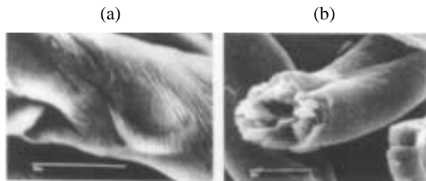
Fig. 1. REM micrographs of MCC sample (sample no. 1): (a) general fiber view, magnification 5000; (b) butt part, magnification 3000.
