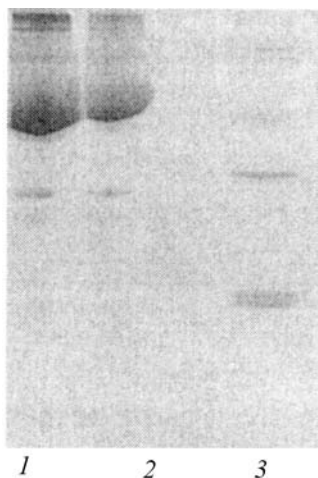
Fig. 2. Electrophoresis in polyacrylamide gel: (1, 2) protein fractions in the permeate and reference, respectively, and (3) markers.
