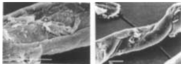
Fig. 5. REM micrographs of cellulose–Ag sample no. 8. Magnification: (a) 2900 and (b) 1600.
